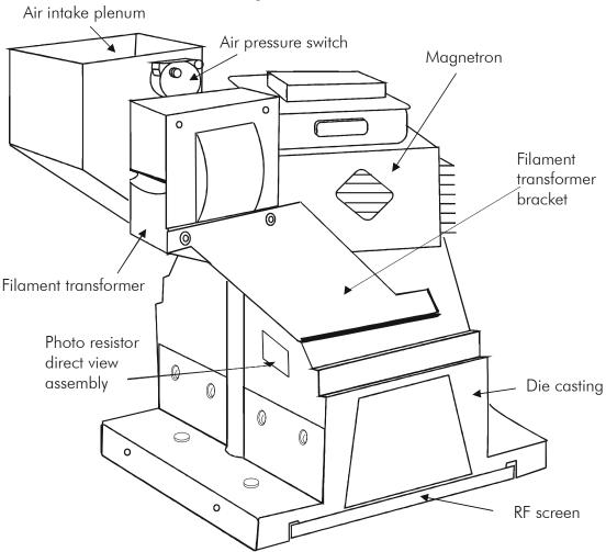
Figure 40. I310M-D/I311M-D Irradiator Component Location (Direct View)
